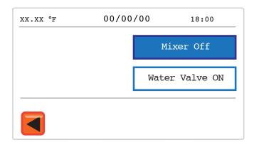
This will call for cooling water to fill the water jacket of the pasteurizer. It may take several minutes for the water jacket to fill with water.
