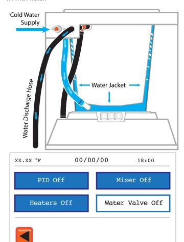
This step will not be necessary in future uses unless the tank is drained. The water valve will open and close as needed while in operation.
